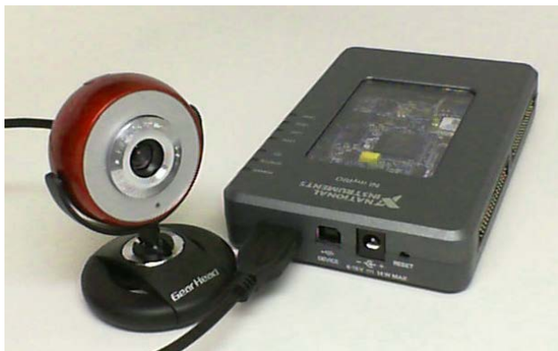
Figure 36.1: webcam connected to NI myRIO USB port.
