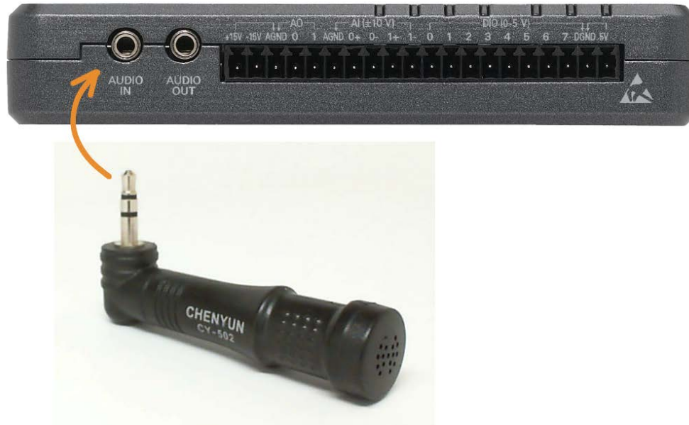
Figure 10.2: Demonstration circuit for electret microphone connected directly to AUDIO IN.
