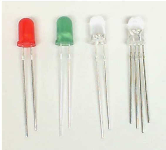
Figure 2.1: Typical LEDs including standard red and green, high-efficiency in various colors, and RGB.
